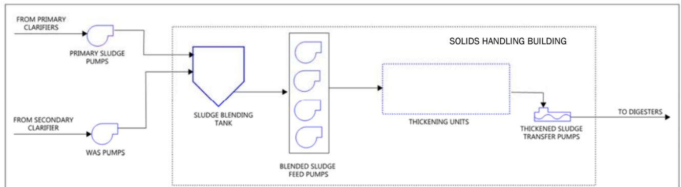
Figure 2. Process flow diagram for Co-thickening (Alternative 4) all housed in the Solids Handling Building
