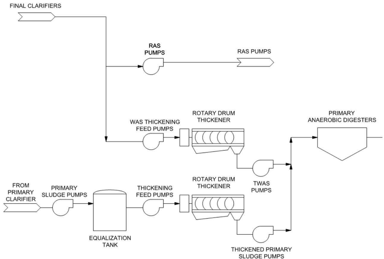
Figure 1. Process flow diagram for separate WAS thickening in the SHB and PS thickening in a new building as in Alternatives 1 through 3 (showing RDTs for PS thickening per Alternative 1)
