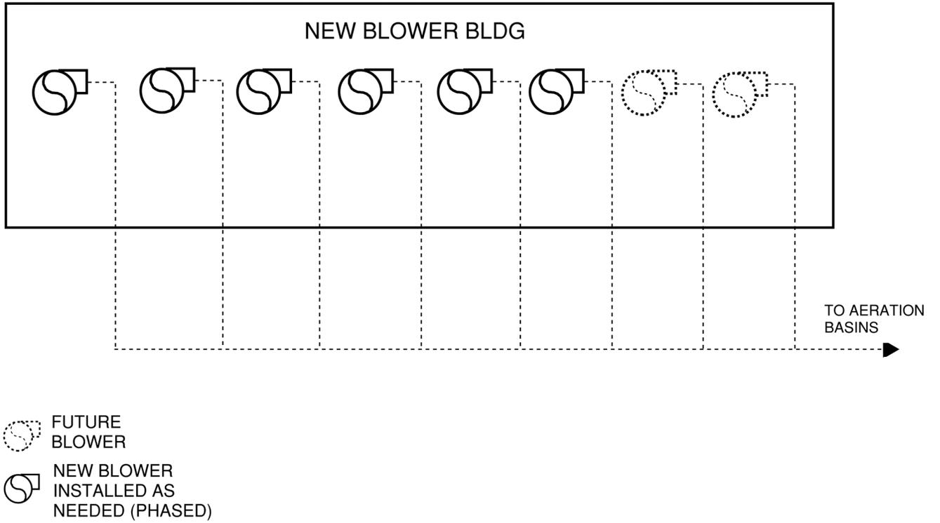
Figure 5. Process flow diagram—Alternative 5
