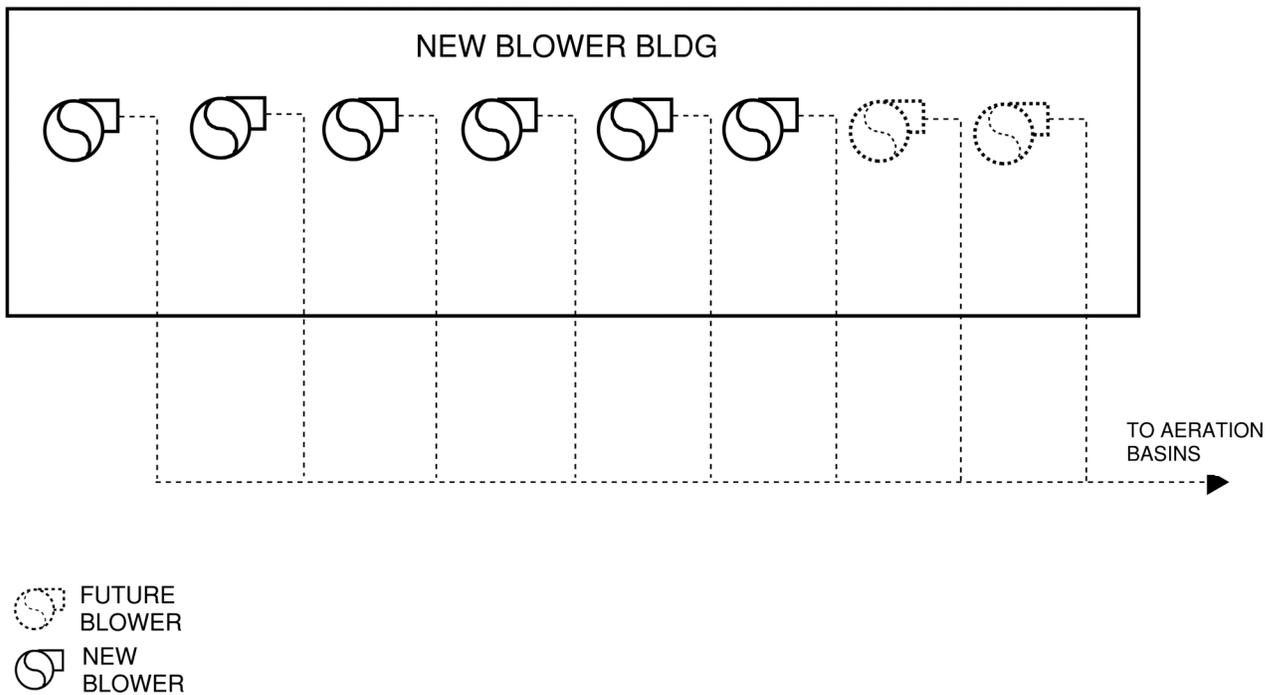
Figure 4. Process flow diagram—Alternative 4
