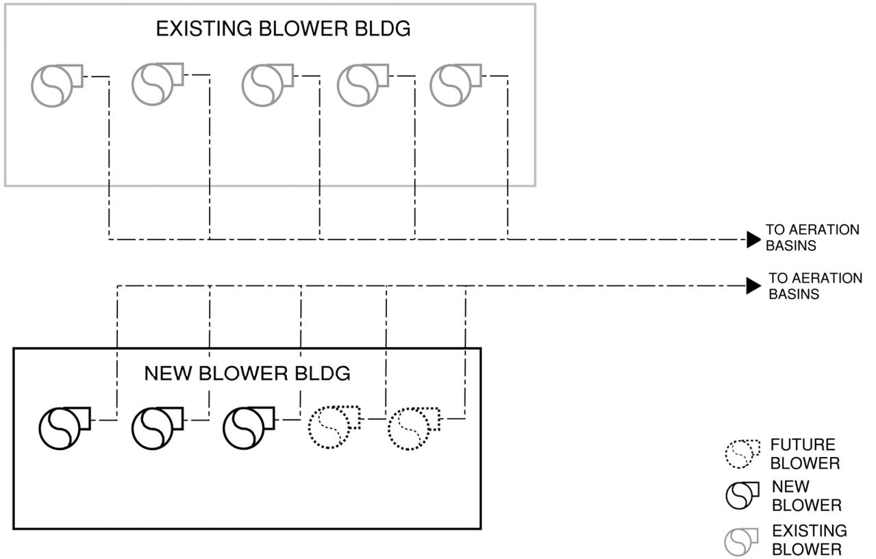
Figure 3. Process flow diagram—Alternative 3
