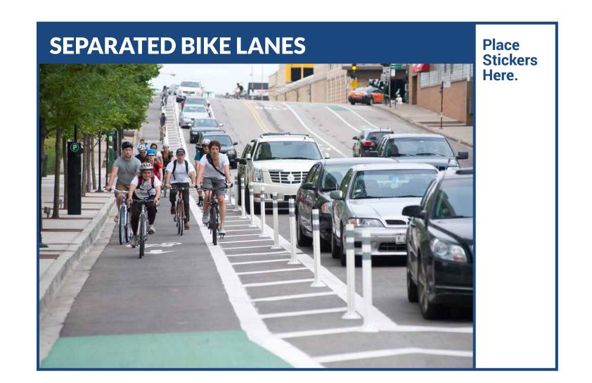
Separated bike lanes are separated from motor vehicle traffic by a physical barrier and not just paint. Barriers may include bollards, concrete planters, or curbs.
