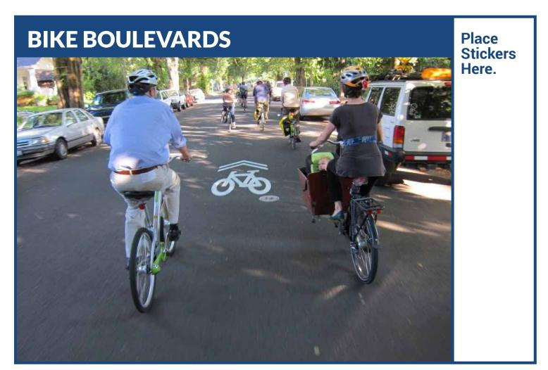
Bike boulevards are low-volume/speed streets modified to enhance bicyclist comfort by using signage, pavement markings, traffic calming and/or traffic reduction, and intersection modifications.
